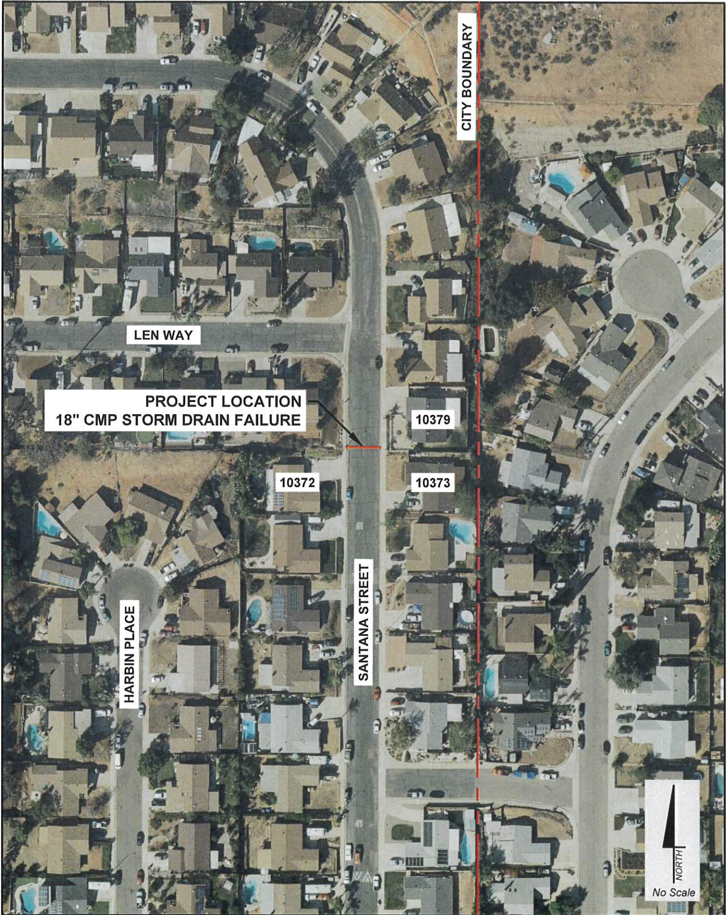
CMP STORM DRAIN - SANTANA STREET EXHIBIT A
