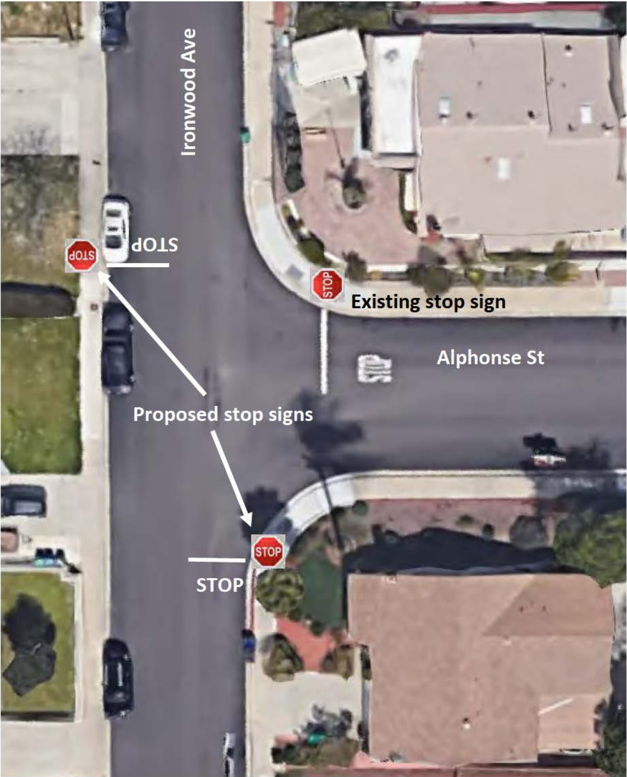
stop sign, legend, and stop bar location.
