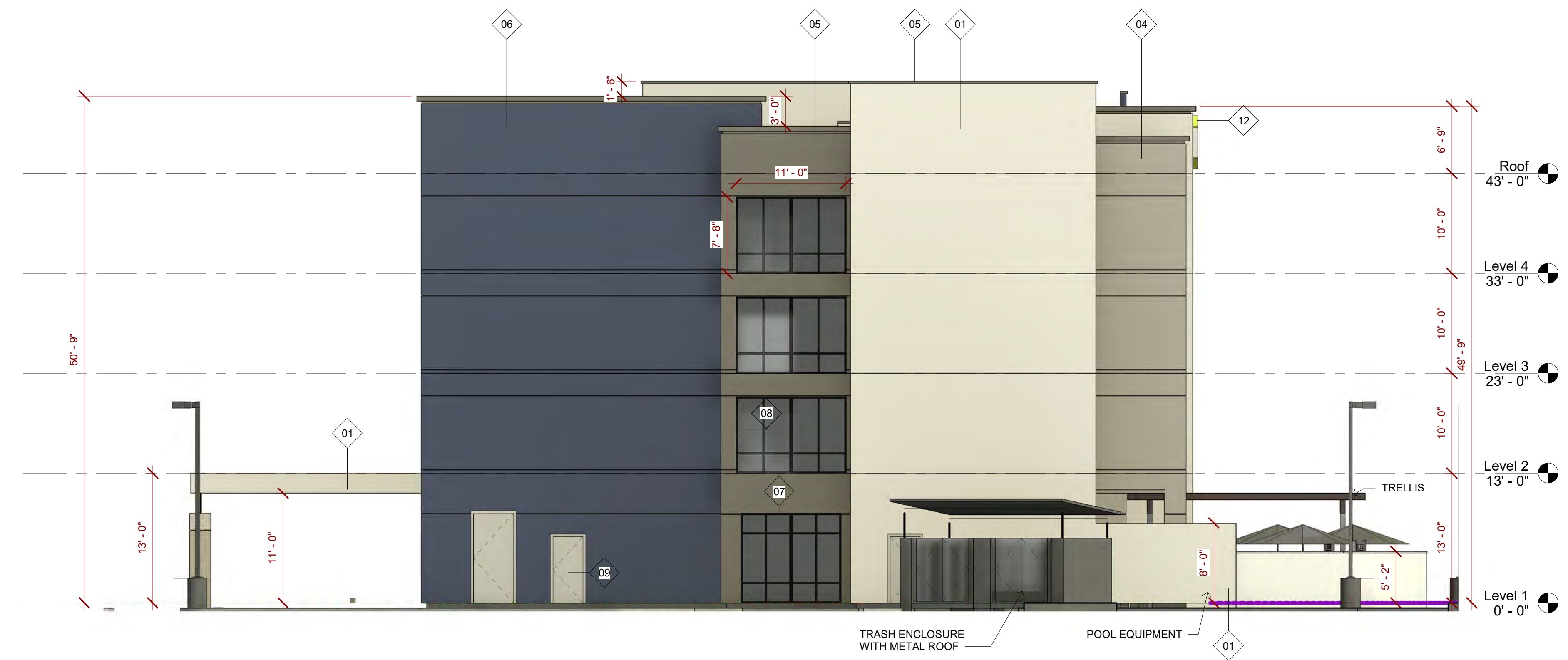
1 South Elevation A-9 1/8" = 1'-0"
