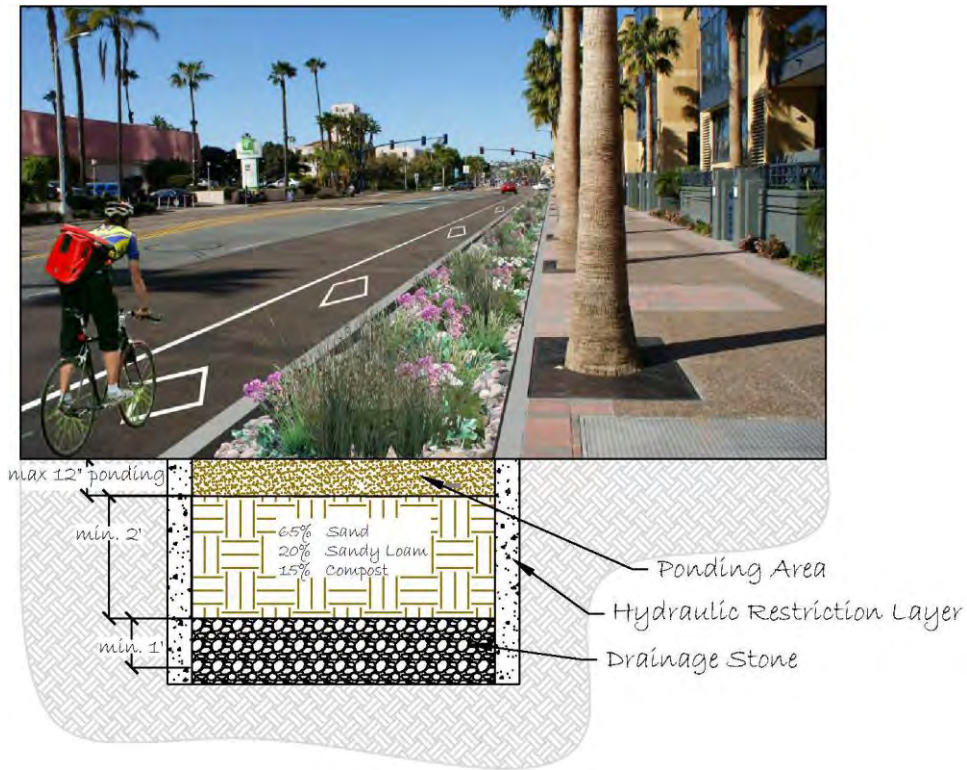
Figure A.11-9. Lateral hydraulic restriction layer.
