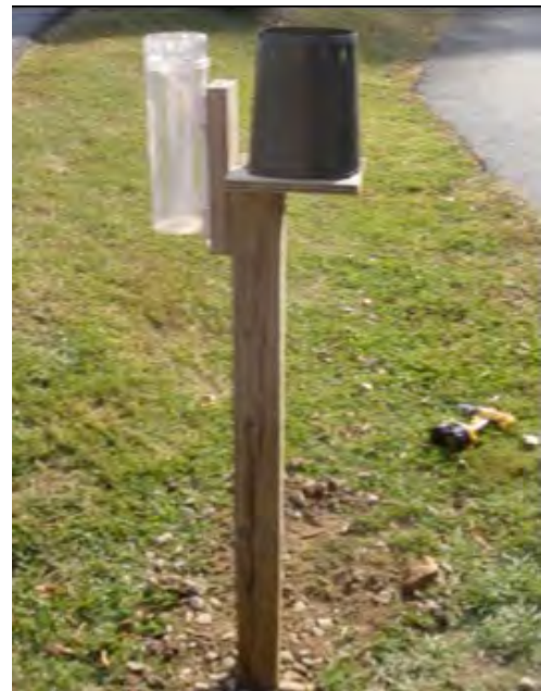
Figure 4-19. Example of manual (left) and tipping bucket (right) rain gauges.
