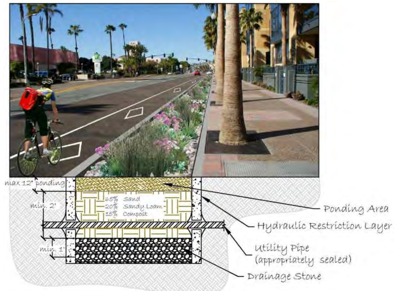
Figure A.11-11. Utility through a hydraulic restriction layer.
