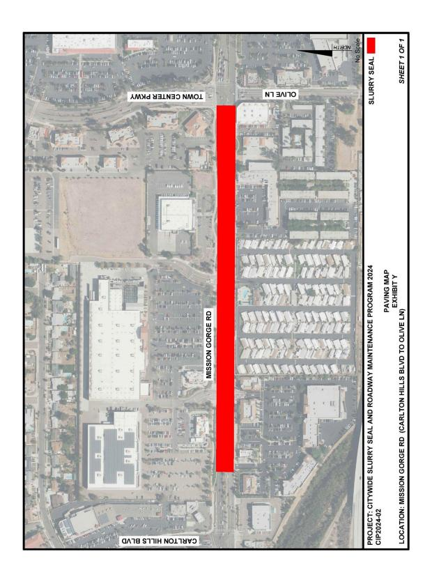
Mission Gorge Rd - Paving **EXHIBIT Z**Citywide Slurry Seal and Roadway Maintenance Program 2024
