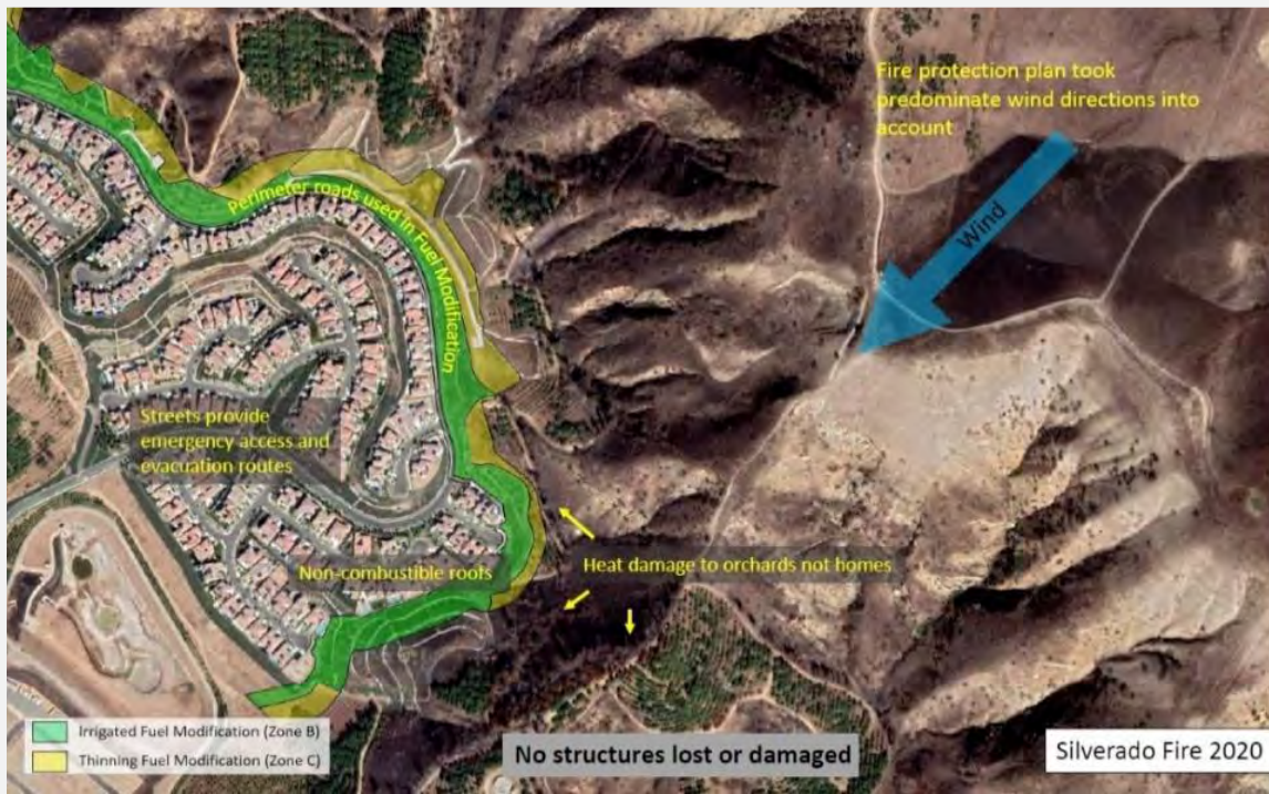
Exhibit 6. 2020 Silverado Fire. Despite extreme fire weather conditions and open space fuel, no homes were damaged or lost in the new, fire hardened community protected by perimeter FMZs and ignition resistant structures.
