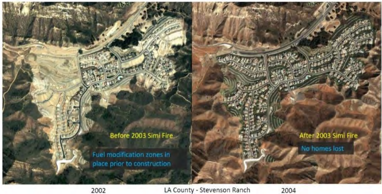
Exhibit 4. 2003 Simi Fire. Note the location within an open space preserve and the wide FMZs surrounding ignition resistant structures. No homes were lost during the 2003 wildfires that threatened the community, and residents remained on site during the event
