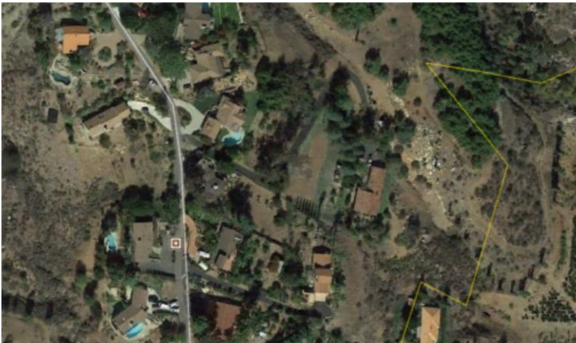
Figure 7. Example of moderate density development. Homes are located on larger properties and include varying levels of ignition resistance and landscape / fuel modification provision and maintenance. This type of development results in a higher wildland exposure level for all homes and does not provide the same buffers from wildfire encroaching onto the site, or starting at a structure and moving into the wildlands as a higher density project.
