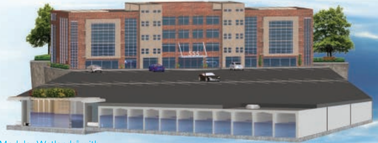
Modular Wetlands® with Box Culvert Prestorage
