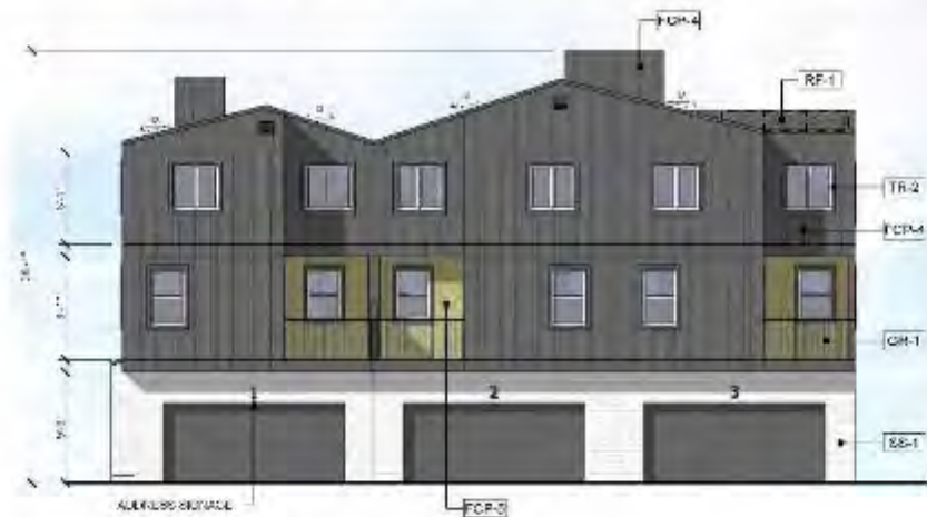
BUILDING 3 - SOUTH ELEVATION SCALE: 1/8" = 1'-0"
