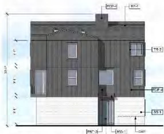
BUILDING 3 - EAST ELEVATION SCALE: 1/8" = 1'-0"
