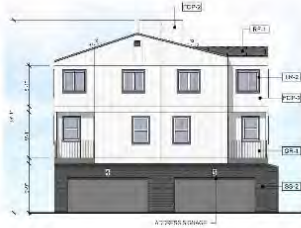
BUILDING 2 - SOUTH ELEVATION SCALE: 1/8" = 1'-0"
