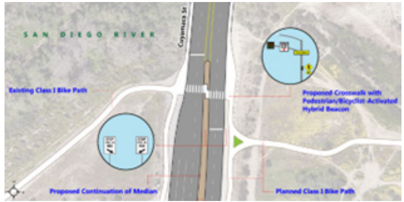
Figure 3-17: Pedestrian/bicycle-activated crosswalk across Cuyamaca Street.
