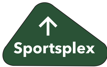
SIGN PANELS FACES: DARK GREEN BACKGROUNDS WITH WHITE REFLECTIVE TYPE (TYPICAL FOR ALL SIGNS)
