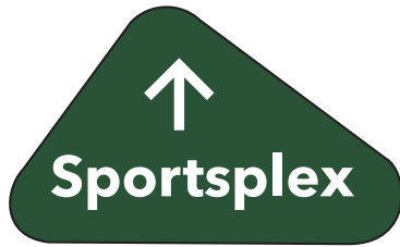
SIGN PANELS FACES: DARK GREEN BACKGROUNDS WITH WHITE REFLECTIVE TYPE (TYPICAL FOR ALL SIGNS)
